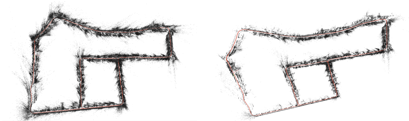
Figure 1. (left) original reconstruction of map (right) reconstructed map with outliers rejection by removing large uncertainty map points
